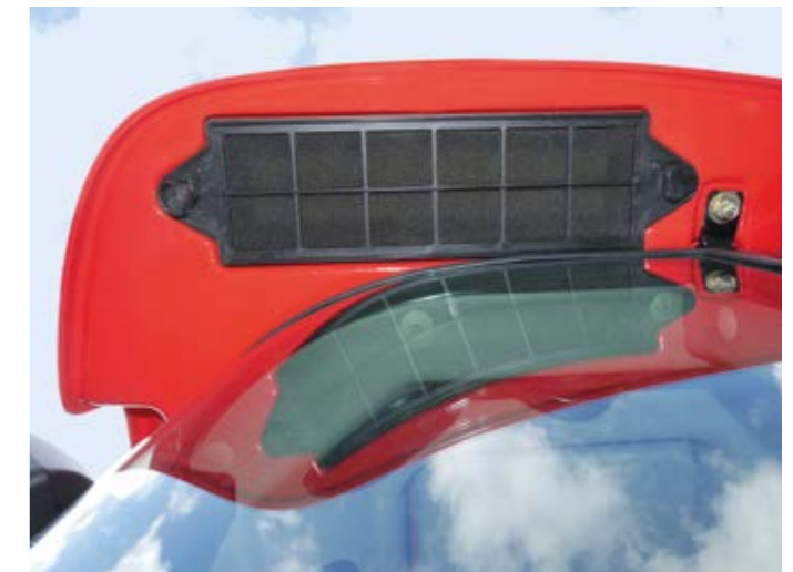
Operating filters and fluids are easily available without the need for special tools.
