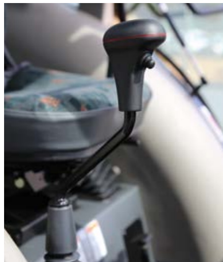
The joystick to control the front loader and attached machines is standard on every tractor.
