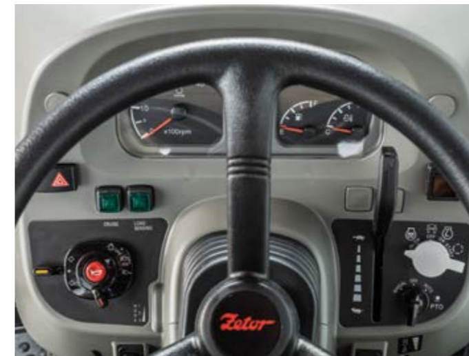
The easy-to-read LED dashboard displays basic operating data, such as engine speed, temperature, fuel level, time, PTO, etc.
