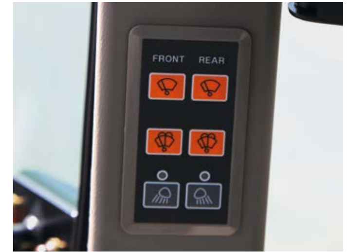
The control panel for lights and wiper is located on the right column so that all buttons are within easy reach of the driver.
