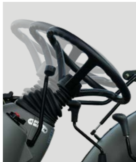
The adjustable steering wheel allows easy access and exit from the cab.
